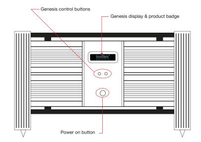
The IsoTek Genesis completely re-defines the term mains regeneration. IsoTek believe it to be the first true mains generator. The mains sine wave is not corrected (as in other devices) but totally and completely rebuilt, 'generated' from new with a THD distortion figure of less than 0.3%. More over it has two generation engines.
