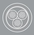
EV03 Sequel refines the multi-strand geometry of Premier as well as incorporating an active shield. The standard fixed length is also increased by half a meter to two meters.
