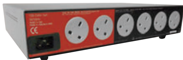
The two sockets (16Amp) in the red coloured area are for high power components such as amplifiers, while source components use the four lower power (10Amp) sockets in the black section. The IEC mains input is on the left."
