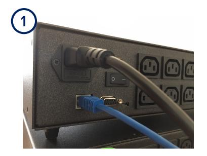
After unboxing your IsoTek SMART power product, please connect the power cord and LAN Ethernet cable, this being connected directly to your router. Connect components to the output sockets via the power cables provided.
