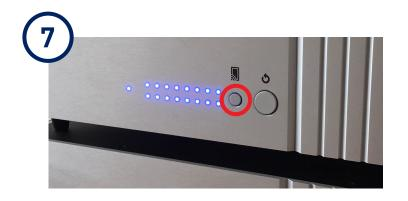
Once the 'PAIR' button has been pressed within the on-line control environment the SMART power front panel lights will start to flash. At this point press the small 'Pair' icon button on the front of the SMART power unit to connect your IsoTek product to the on-line control interface.
